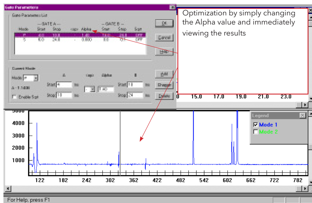
Figure 5.4. Post-Run Optimization of Gate Alpha Values
