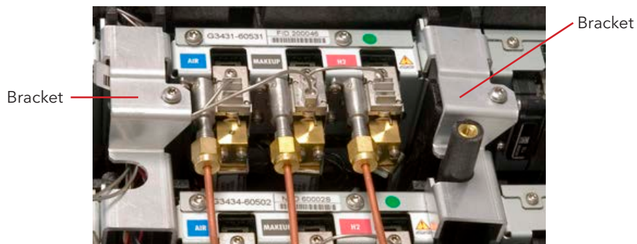
Figure 3.21. Locating the EPC Module Brackets
